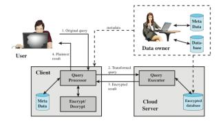
Figure: Encryption scheme for a cloud-based Database [1]
