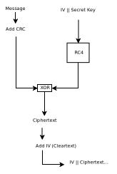
Figure: WEP encryption process
